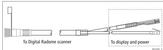
For Digital Radome scanners that are purchased with a cable, the length should be sufficient to complete the cable run on most small boats. For longer runs, and for Digital Radome scanners that are purchased without a cable, optional cables and extension cables are available.
