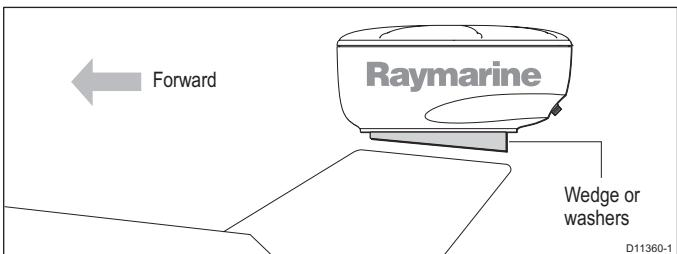
Planing hull and some displacement hull boats adopt a higher bow angle when the boat is at cruising speed, giving poor target detection. It may be necessary to lower the radar beam back towards the parallel, by shimming the rear of the radar, so that the beam points slightly down when the boat is at rest. Refer to the diagram on page 14 for more information.
