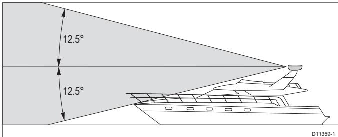
Mount the scanner so that the array rotates parallel to the waterline. The radar beam is approximately  $25^{\circ}$  wide in the vertical direction, giving good target detection when your boat pitches and rolls.
