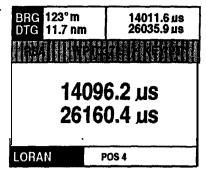
Note also, that the sensor mode in use here is the Loran-C. The NAV 398, when operating in the GPS mode can convert the GPS **Lat/Lon** readouts into **GPS/Loran** Time Differences (TDs). Some users may find this calculation useful to reference with their old loran coordinate logs.
