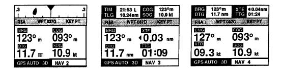
Generally, the NAV screens are more useful once a **waypoint** has been entered into the units' memories . Once a **waypoint** destination is selected, the **NAV1** display will feature large readouts of the destination Bearing **(BRG)and** Distance-to-go **(DTG)** to the **waypoint** combined with the Course and Speed readouts. The readouts in the upper section of the display show the XTE,TTG, local time, and trip log distance.
