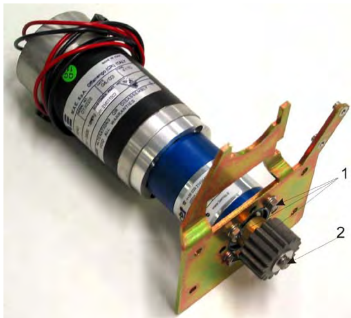
Figure: 4-59 Antenna rotation motor
