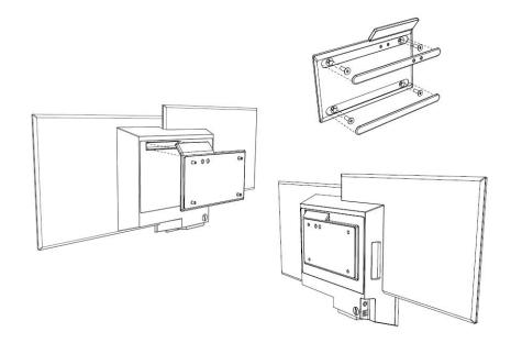
NOTICE: The ELECTROSTATZ<sup>™</sup> tweeter panels, LHS & RHS, are dipole i.e. sound waves travel in both directions. To maintain the highest quality acoustic performance, never block the rear sound output area and always maintain at least a 3cm distance between the tweeter panels and the wall. The mounting bracket will automatically provided the clearance required
