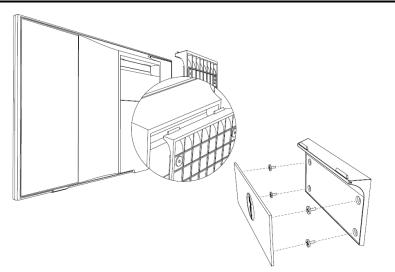
NOTICE: The ELECTROSTATZ™ tweeter panels, LHS & RHS, are dipole i.e. sound waves travel in both directions. To maintain the highest quality acoustic performance, never block the rear sound output area and always maintain at least a 3cm distance between the tweeter panels and the wall. The mounting bracket will automatically provided the clearance required
