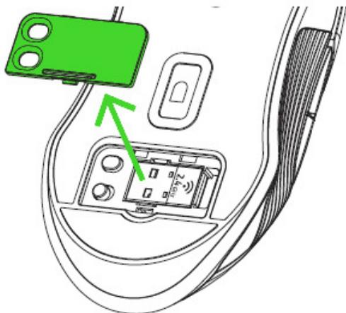
2. Remove the USB wireless receiver from your PC and place it into the storage space.
