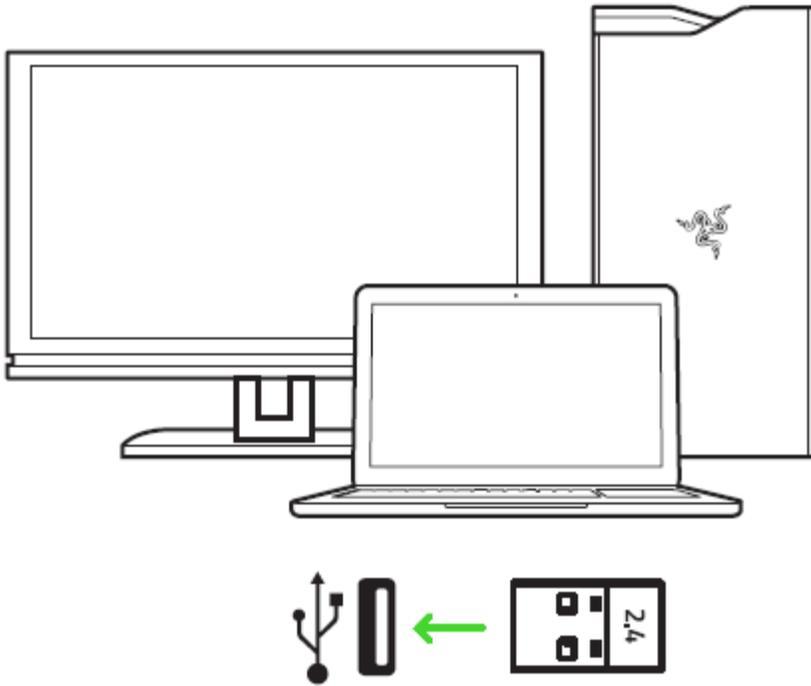
Step 1: Make sure the USB wireless receiver is connected to the USB port of your computer.
