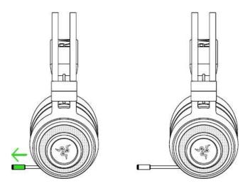
Bend the mic until it is parallel to your mouth, then adjust the length as preferred. Make sure the mic diaphragm is in front and the air vent is facing away from your mouth.
