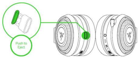
**Note:** To return the USB wireless transceiver, push it into the compartment until you hear a click.
