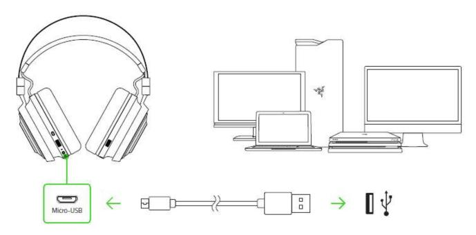
For best results, please fully charge your headset before using it for the first time. A depleted unit will fully charge in about **4 hours**.
