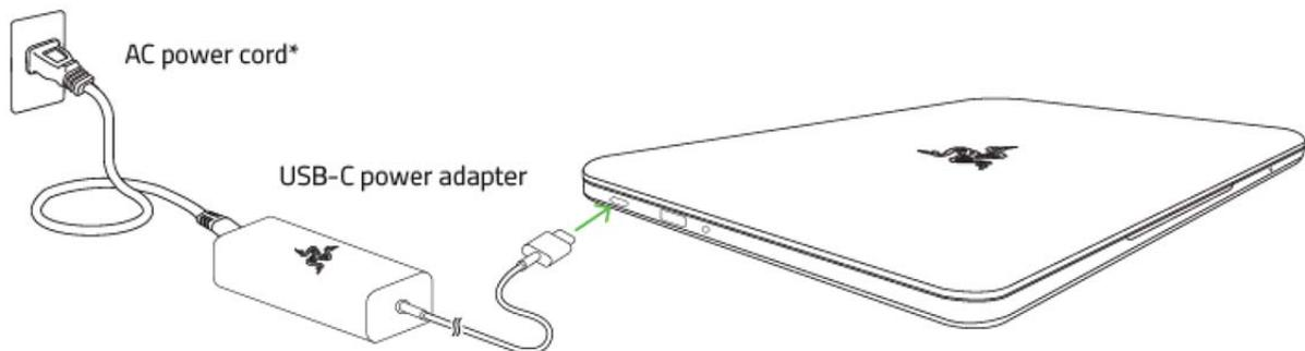
Make sure that the AC plug is properly inserted into the power outlet and the power adapter. Insert the power adapter's USB-C connector into any of the Razer Blade Stealth's power ports. Press the power key to turn on your Razer Blade Stealth.
