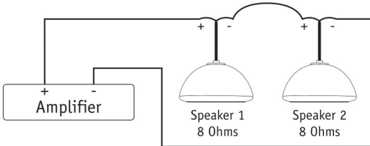
In this example, each speaker has an impedance of 8 Ohms. In a series connection as shown here, the total impedance equals  $8+8$  or 16 Ohms. The total impedance of a series connection is the sum of each speaker's impedance.
