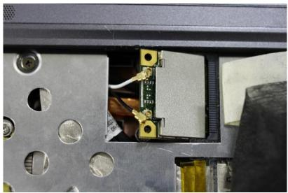
Step 3. Remove the Wireless PCle MiniCard module board from PCle MiniCard connector port.
