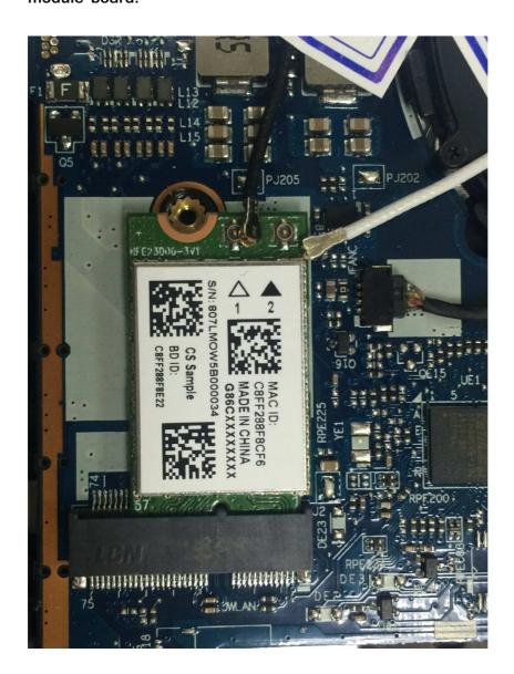
Step 3. Remove the Wireless PCle NGFF1630 module board from PCle
