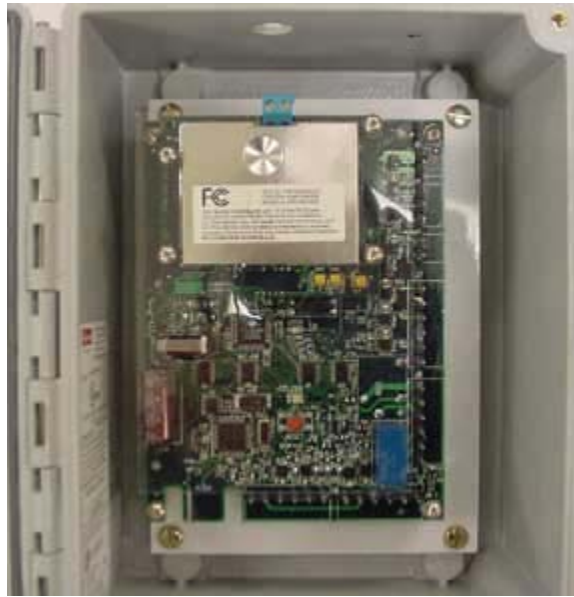
Figure 5-17 – Replacing the WRI's PCB
