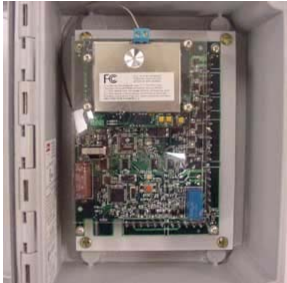
Figure 5-14 – Removing the WRI PCB
