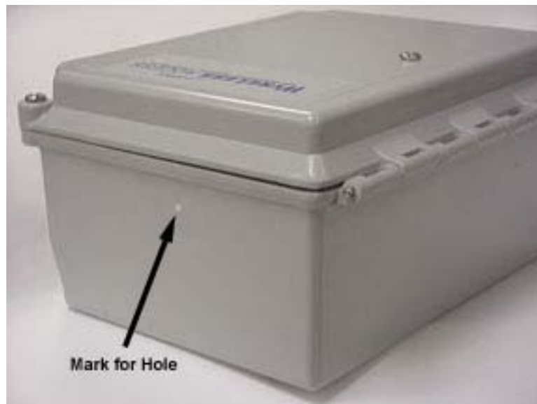
Figure 5-16 – WRI -OTD Antenna Hole Locations
