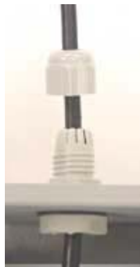
Figure 5-13 – Securing the PIM's Antenna NEMA Gland
