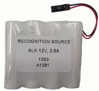
Figure 6-2 – WISI Battery Pack
