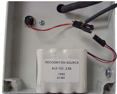
Figure 8-4 – WPR Battery Pack Positioned
