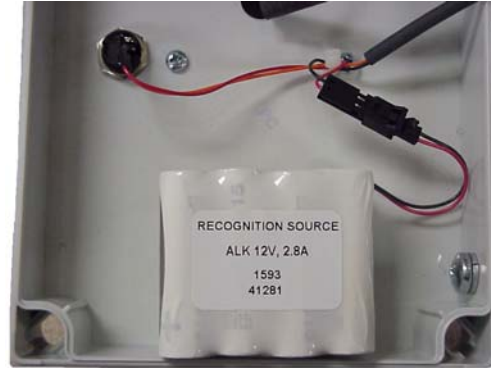
Figure 8-6 – WPR Battery Pack Connected
