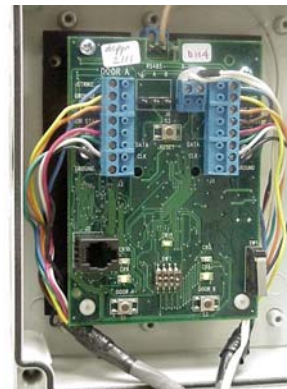
Figure 3-4 – Proper Wire Routing
