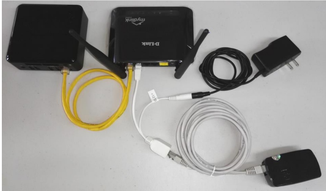
Figure 3 - Connection of the RBS, a POE powered bridge to the Wi-Fi router
