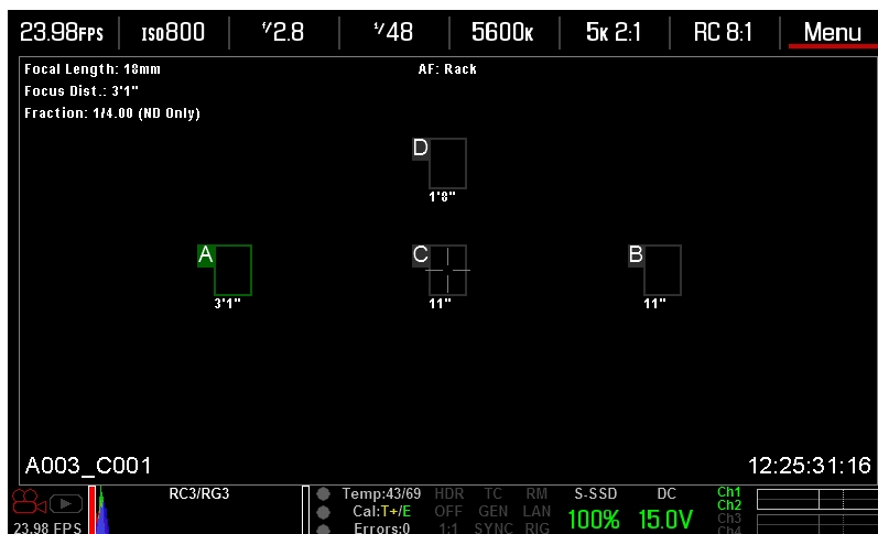
Figure: Set Rack Point Location
