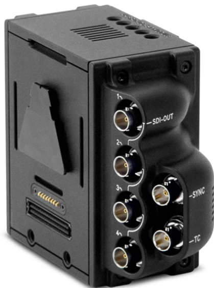
Figure: REDCAST Module
