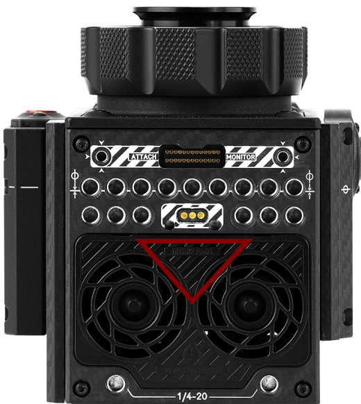
Figure: Do Not Obstruct WiFi Antenna
