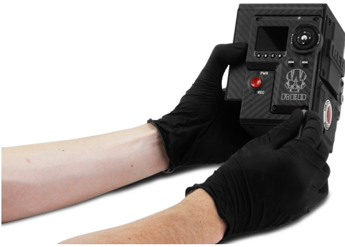
Figure: Remove DSMC2 Sidekick
