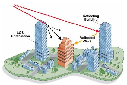
Figure 6: System - Non-Line of Sight Deployment
