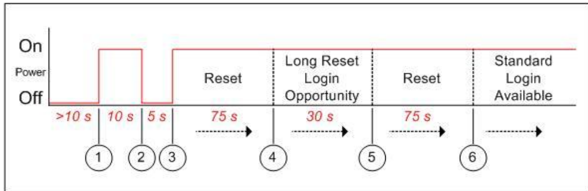
Fig. 63: Diag. - Recovering Lost IP Address
