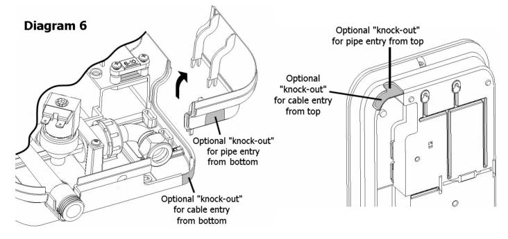
5. Decide the position of the electrical cable into the unit. If top or bottom entry is chosen (according to diagram 4), cut away the walls in the backplate as shown in diagram 6.
