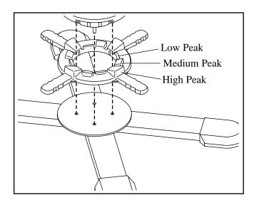
MEDIUM STABILITY (INTERMEDIATE): Turn the adjustment ring so that the medium-sized peaks on the adjustment ring are positioned directly below the black blocks that extend down from the underside of the top of the board. In this position, the Reebok Core Board is at the middle of the range of resistance/stability.
