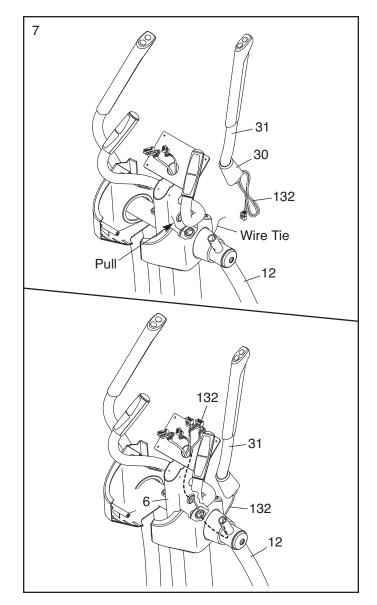
Tip: Avoid pinching the wire. Attach the Right Upper Body Arm (31) to the Right Upper Body Leg (12) with two 5/16" x 1 1/2" Button Bolts (73) and two 5/16" Locknuts (106). Make sure that the Locknuts are in the hexagonal holes.
