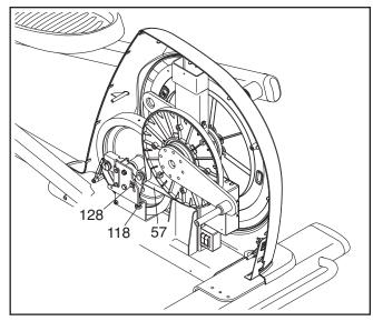
When the Drive Belt (57) is tight, tighten the Pivot Screw (128).
