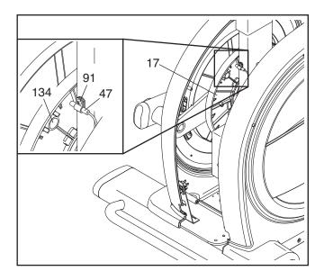
Rotate the Large Pulley (17) for a moment. Repeat these actions until the console displays correct feedback.
