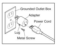
temporary adapter should be used only until a properly grounded outlet can be installed by a qualified electrician.
