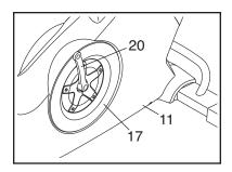
Rotate the left Pedal Disc (17) clockwise to release it from the Left Shield (11).
