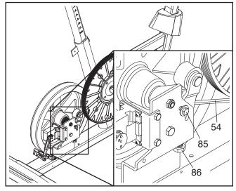
When the Drive Belt (54) is tight, tighten the M6 x 20mm Hex Screw (85).
