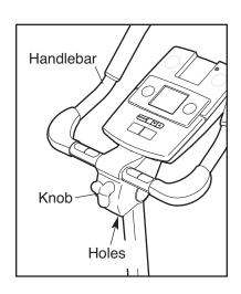
adjustment holes. Then, tighten the knob.
