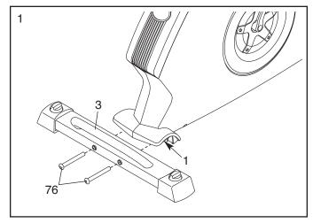
2. Attach the Front Stabilizer (2) to the Frame (1) with two M10 x 95mm Patch Screws (76).
