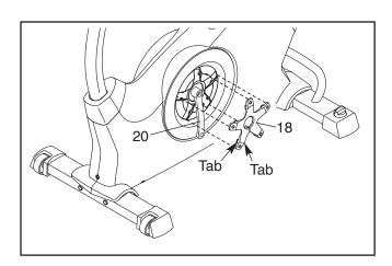
Using a flat screwdriver, release the tabs on each point of the left Disc Cover (18). Carefully work the left Disc Cover over the Left Crank Arm (20) and remove the left Disc Cover.
