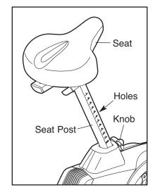
knob is engaged in one of the adjustment holes in the seat post. Then, tighten the knob.
