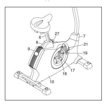
Using a flat screwdriver, remove the Top Shield Cover (8) and the Rear Shield Cover (9). Then, use the flat screwdriver to release the Front Shield Cover (7).
