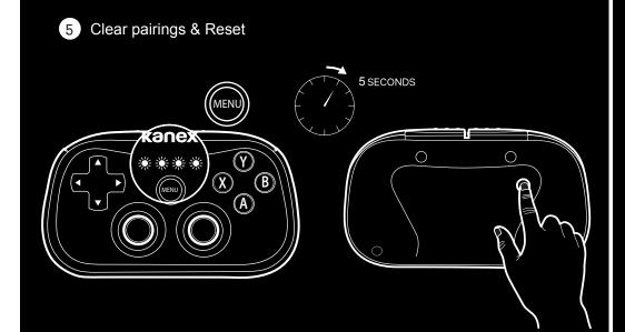
Pressing and holding both the munu button and Bluetooth button simultaneously for 5 seconds to clear all saved Bluetooth pairings. This may also to reset the controller.
