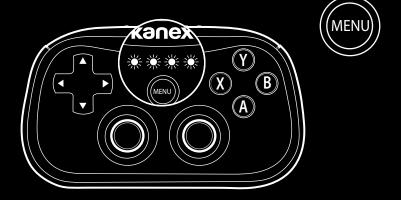
Pressing and holding the menu button for 0.6 seconds to power on the controller from an off state.
