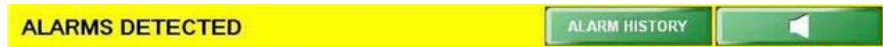
Figure 5-10. Yellow Alarm Status bar with ALARM HISTORY and Alarm Silence buttons, indicating diagnostic alarms
