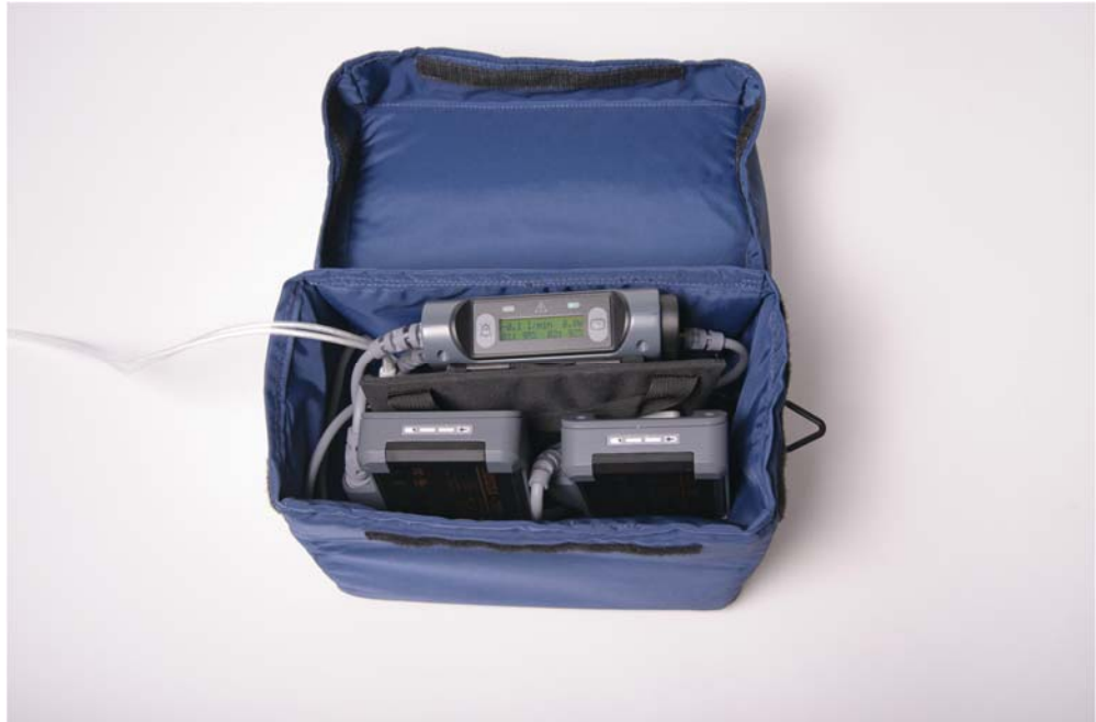
Figure 6-3. Properly inserting the Controller, battery pockets, batteries, and cables in the VADPAK Insert into the shower bag
