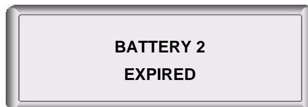
Figure B-20. Diagnostic alarm 10: BATTERY 2 EXPIRED
