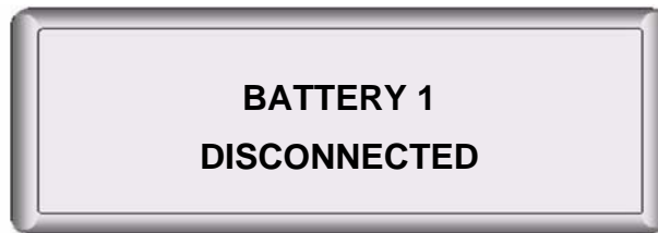
Figure B-15. Diagnostic alarm 5: BATTERY 1 DISCONNECTED
