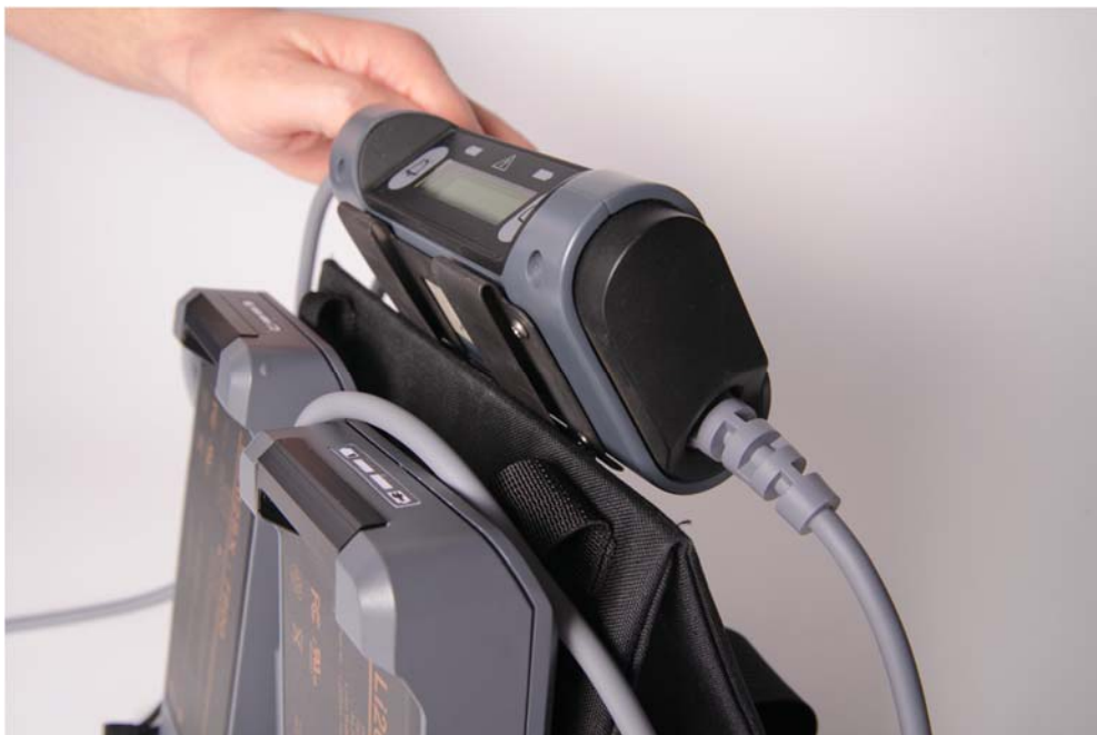
Figure 4-22. Securing the Controller into the VADPAK Insert with the Controller display facing upward
