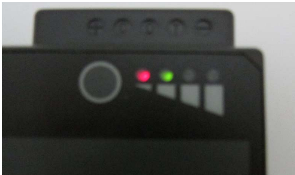
Figure 4-32. Battery charge level indicators
