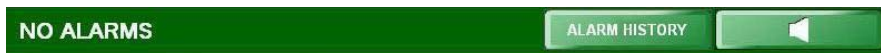
Figure 5-9. Green Alarm Status bar with ALARM HISTORY and Alarm Silence buttons, indicating normal conditions
