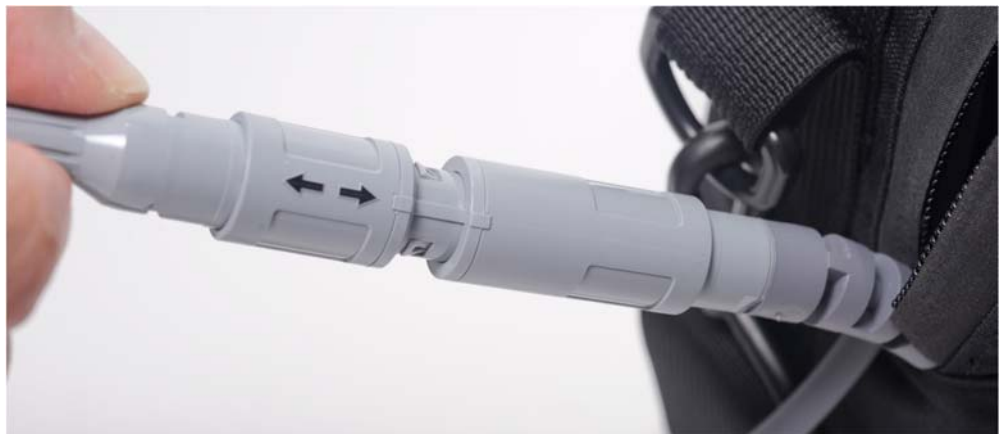
Figure 4-29. Aligning the arrow on the power source connector with the square on the battery pocket external power connector
