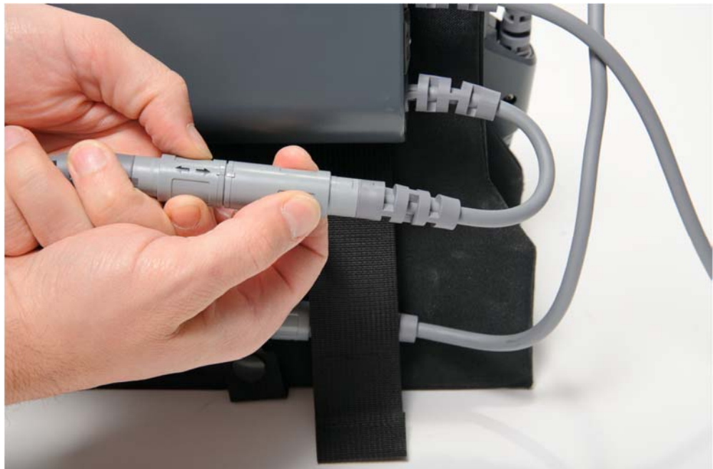
Figure 4-33. Aligning the arrow on the battery pocket connector with the square on the Controller connector
