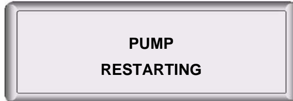
Figure B-14. Diagnostic alarm 4: PUMP RESTARTING
