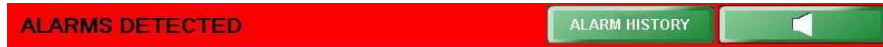
Figure 5-11. Red Alarm Status bar with ALARM HISTORY and Alarm Silence buttons, indicating emergency alarms
