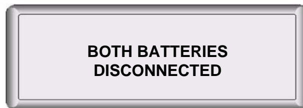
Figure B-9. Emergency alarm 2: BOTH BATTERIES DISCONNECTED
