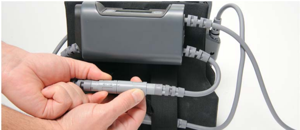
Figure 4-34. Batteries connected to the Controller
