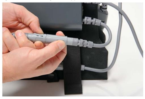
4. Connect the battery pocket to the backup Controller.
