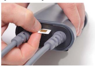
3. Insert the SIM card into the backup Controller.
