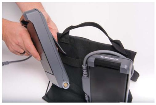
3. Slide the Controller onto the fabric strap using the Controller belt clip so that the Controller display is facing upward.
