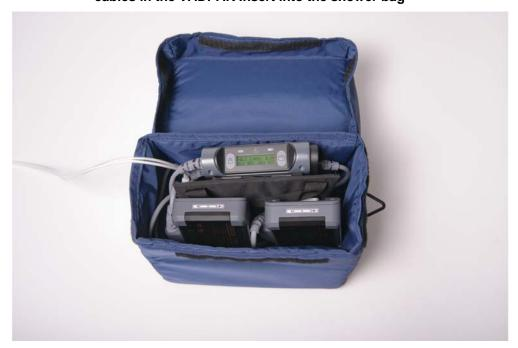
3. Secure the percutaneous cable to the side of the shower bag using the Velcro® strap attached to the left side of the shower bag.
