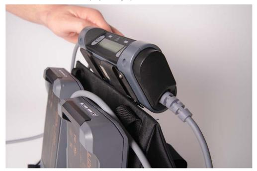
4. Secure the battery connectors and cables below the Controller using the Velcro® straps.
