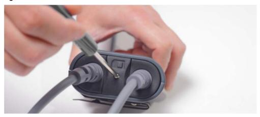
2. Remove the SIM card from the malfunctioning Controller.
