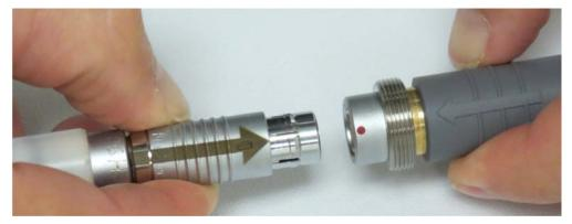
7. Firmly press the connectors together to connect the backup Controller to the VAD. A slight click sounds as the connectors snap into place and become fully seated.
