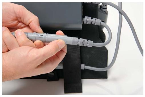
2. After you align the arrow and the square, firmly push the battery pocket connector straight into the Controller connector.
