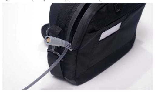
2. Visually align the arrow on the power source connector (such as the Independent Power Supply) with the square on the battery pocket external power connector on the bottom of the battery pocket.
