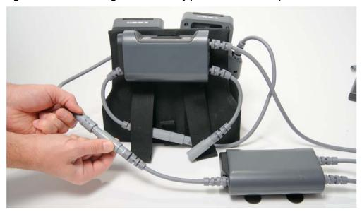
5. Pull the ribbed section of the driveline connector to disconnect it from the malfunctioning Controller.
