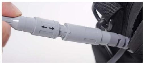
3. Once the arrow and the square are aligned, firmly push the power source connector straight into the battery pocket external power connector.
