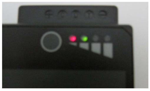
Each battery contains an integrated charge level indicator display consisting of four LEDs on the face of the battery. The LEDs represent the maximum charge level the battery contains in 25% increments. Table 4-1 describes the LED battery charge level indicators.
