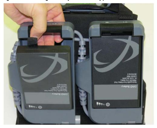
Figure 4-35. Removing the battery from the battery pocket
