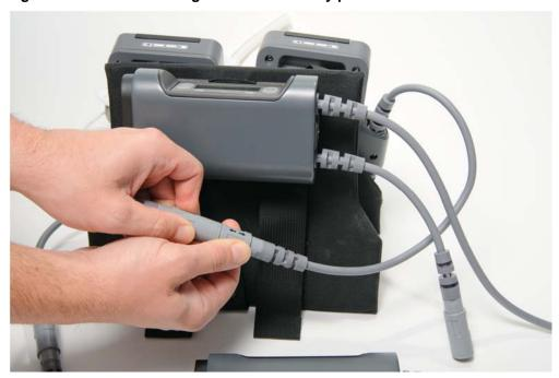
11. Connect the second battery pocket to the backup Controller.
