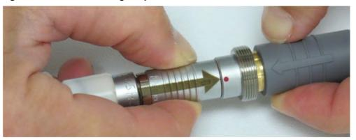
6. Align the arrow on the driveline connector to the groove on the backup Controller connector.
