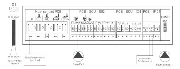
Note: Control PCBs are shown diagrammatically Earths are omitted for clarity
