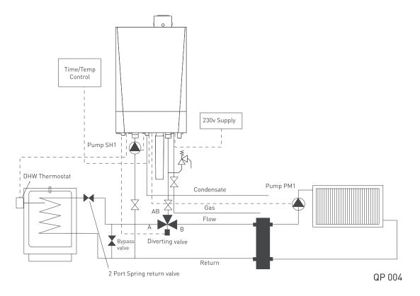
Single Quinta Pro boiler, heating with priority hot water using a low loss header pump option. DHW priority can be used on all Quinta Pro range
