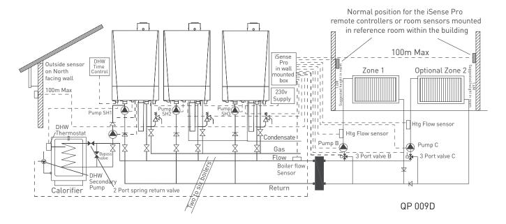
Multiple Quinta Pro boilers, heating and priority hot water using a low loss header, outside weather or room compensation with the iSense controller (Hot water produced by single boiler only - pump option)
