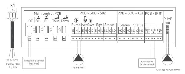
Note: Control PCBs are shown diagrammatically Earths are omitted for clarity
