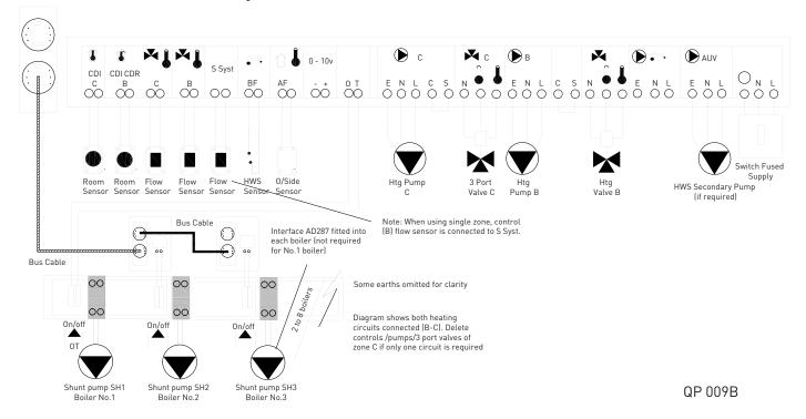
Multiple Quinta Pro boilers, heating and HTG and DHW using a low loss header, outside weather/room compensation with the iSense Pro controller (DHW via multiple boilers) (to be used in conjuction with QP009A)
