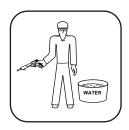
8. Should the tool fail to fire, hold the muzzle firmly against the work surface for 30 seconds. Release the trigger and remove pressure on the tool while holding the muzzle against the work surface. Again press the tool firmly against the work surface and pull the trigger. If the tool still fails to fire, hold the tool firmly against the work surface for another 30 seconds before unloading and carefully discarding the misfired power load into water or oil.
