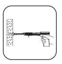
6. Squeeze trigger to set power fastener. Be sure to keep pressure on tool during this operation.
