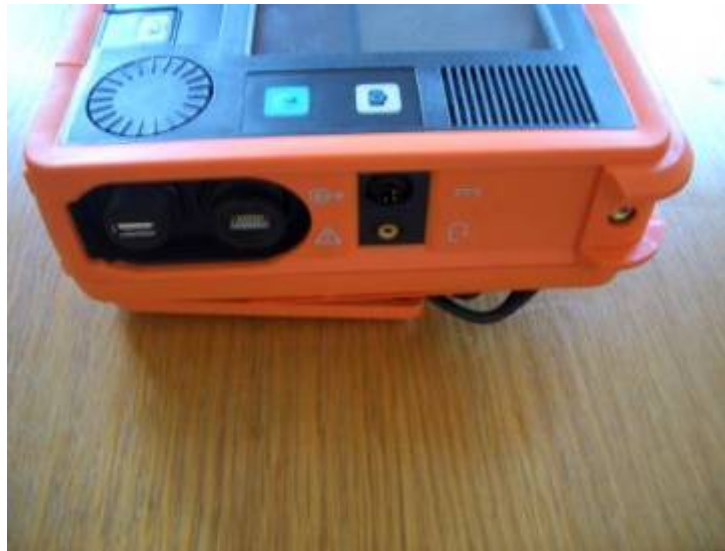
Communications Connection Panel
