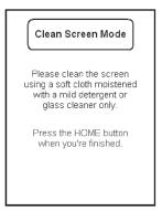
To clean your T2-Cs, lightly dampen a lint-free cloth with a glass cleaner or mild detergent, and wipe the touchscreen, keypad and outer surfaces.
