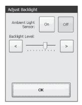
If the light sensor is enabled, there are two backlight levels to adjust. Press the left arrow or right arrow buttons to adjust. Press the OK button when finished.
