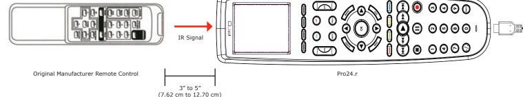
The Pro24, r is capable of capturing infrared codes from original equipment manufacturer remote controls. This IR learning capability is designed to work together with the Pro Control Studio library manager software. To capture infrared codes, follow the steps listed below:
