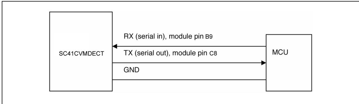
**Figure 6** UART hardware configuration
