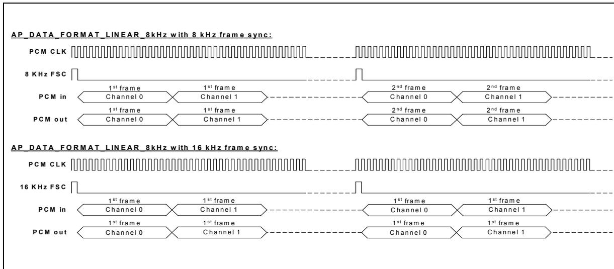
Figure 17 PCM bus with linear PCM, 8kHz sample rate
