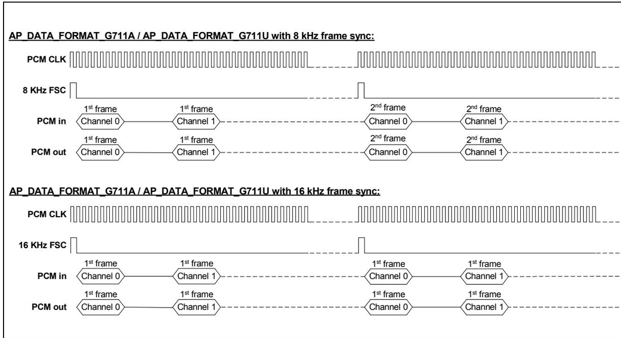
Figure 19 PCM bus with G.711 – A-law/u-law, 8 kHz sample rate
