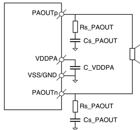
**Figure 8 Loudspeaker connection**
