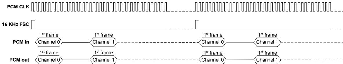
**Figure 21 PCM bus with compressed wideband using A-law/ ?-law, G726 used on air interface.**
