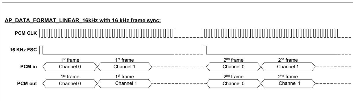
Figure 18 PCM bus with linear PCM, 16kHz sample rate
