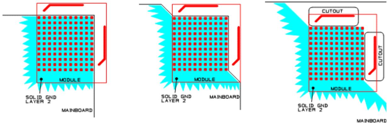
Figure 28 Module placement on the main board (top view)
