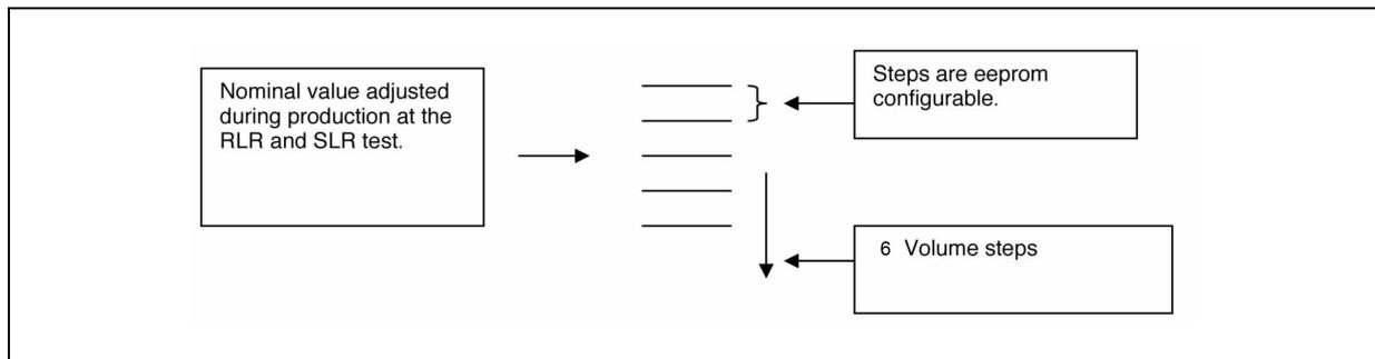
Figure 10 Handset Volume Configuration
