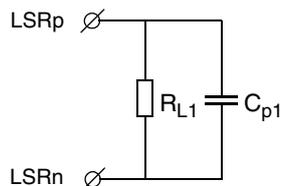
**Figure 22 Load circuit A Dynamic loudspeaker**
