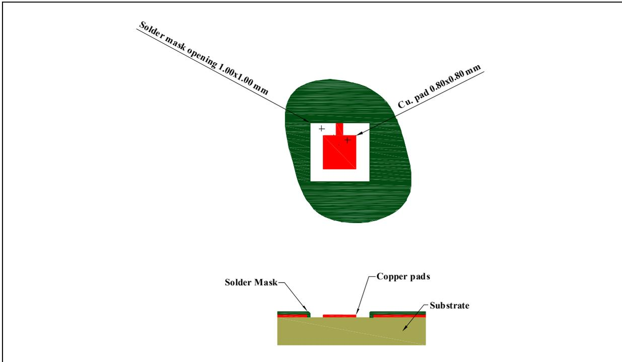
Figure 30 Copper pad and Solder mask opening
