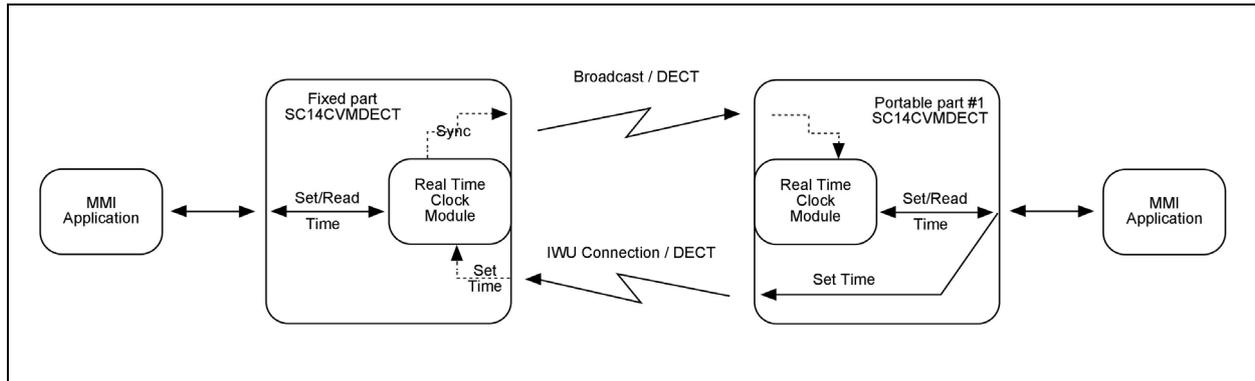
**Figure 12 Clock synchronization**
