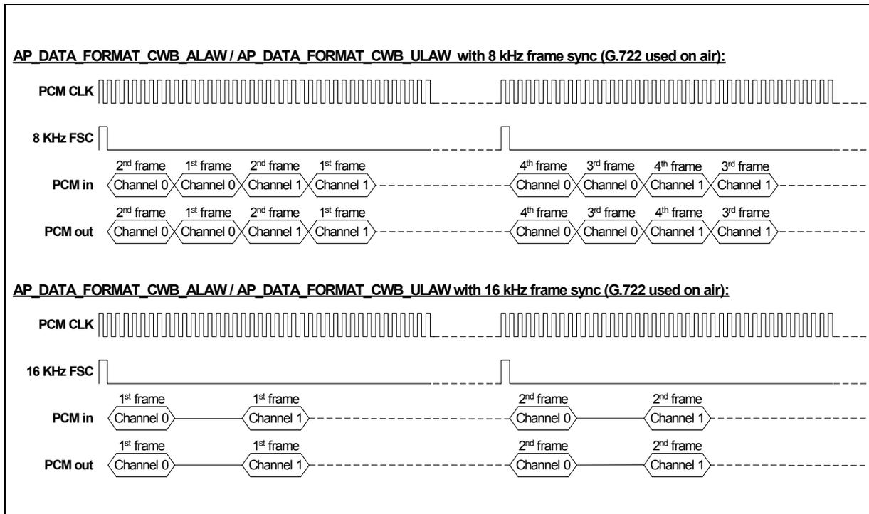
Figure 20 PCM bus with compressed wideband using A-law/ u-law, G722 used on air interface.
