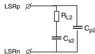
**Figure 23 Load circuit B Piezo loudspeaker**
