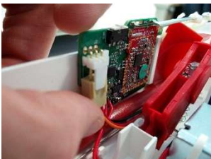
Remove the battery connector
