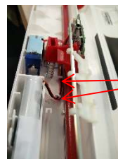
Hook the cable under the clips
