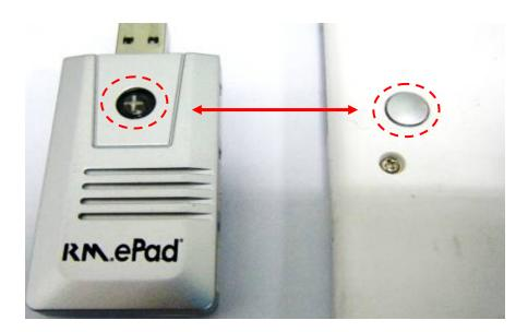
Red LED on power button will flash (2-3 times) and then light up continuousely.
