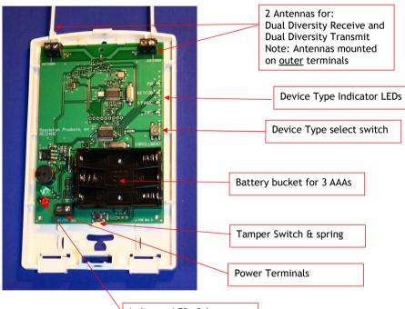
Indicator LEDs & buzzer
