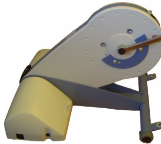
Figure 3: Base unit of the ergometer
