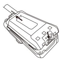
Insert the top part of the battery pack into the top 2 slots of the transceiver and then press the battery pack down until a "click" sound is heard.
