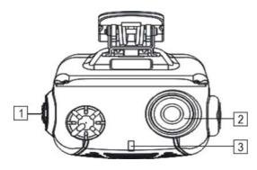
1Power/Volume Knob: Rotate it to turn on the transceiver and to adjust the volume.
