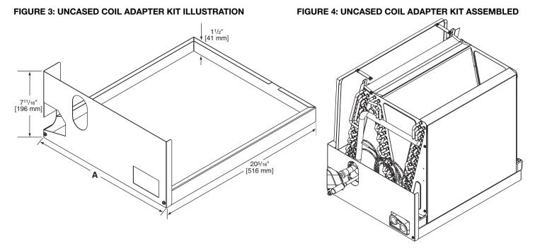
Note: Sliding the coil into the coil rail before attaching coil rack front.
