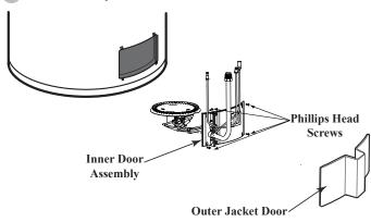
Remove the six phillips screws on the inner door using a phillips screwdriver. Disconnect burner supply tube using the 3/4" wrench, pilot tube using the 7/16" wrench, and thermocouple using the 3/8" wrench from the thermostat. Disconnect the piezo wire from piezo ignitor striker connection. Remove the entire burner assembly along with the inner door.Remove the phillips head screw that holds the pilot burner assembly in place.
