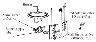
**9** Remove the compression nut from the pilot burner assembly using the 3/8" and 5/16" wrench to expose pilot burner orifice. Remove natural gas pilot burner orifice and replace with **Yellow marked LP pilot burner orifice** supplied in the package. Replace the compression nut on pilot burner assembly and tighten the nut.
