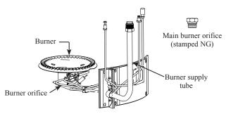
9 Remove the compression nut from the pilot burner assembly using the 3/8" and 5/16" wrench to expose pilot burner orifice. Remove the yellow marked LP gas pilot burner orifice and replace with natural gas pilot burner orifice supplied in the package. Replace the compression nut on pilot burner assembly and tighten the nut.
