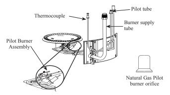
Exploded View of Pilot Burner Assembly
