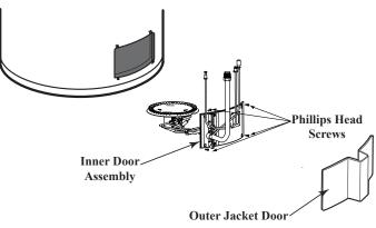
Remove the six phillips head screws on the inner door using the phillips screwdriver. Disconnect burner supply tube using the 3/4" wrench, pilot tube using the 7/16" wrench, and thermocouple using the 3/8" wrench from the thermostat. Disconnect the piezo wire from piezo ignitor striker connection. Remove the entire burner assembly along with the inner door.
