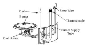
Remove the phillips head screw that holds the pilot burner assembly in place. Remove the pilot burner assembly from the burner bracket. Remove the two #6 x 3/8" long Philips head screws from the burner bracket and remove the burner from inner door assembly to expose main burner orifice.
