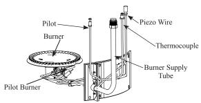
Remove the philips head screw that holds the pilot burner assembly in place. Remove the pilot burner assembly from the burner bracket. Remove the two #6 x 3/8" long philips head screws from the burner bracket and remove the burner from inner door assembly to expose main burner orifice.
