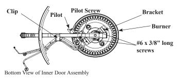
Remove LP burner orifice. Replace Red marked LP gas burner orifice with the main burner orifice stamped NG supplied in the bag.
