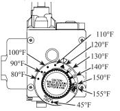
The illustration at the left details the approximate water temperature for each mark on the Gas Control (Thermostat) Temperature Dial.
