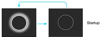
The LED will fade from red to white when the RS485 connection is down or if the reader is not connected to an Access Control Unit (ACU). **ERR: No ACU**
