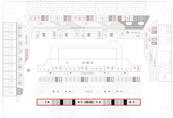
Power to the reader can be supplied directly by the 12VDC power supply in the “WIEGAND” section of the DC20 Door Controller. Alternatively, an external power supply can be used. Note that DR20 requires 8-28VDC with a maximum power of 4.8W. Refer to Recommended Wire Type and Size table above for more wiring detail.
