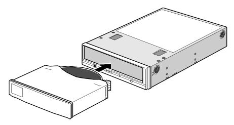
Fig. III -7 How to insert the magazine
