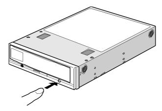
Fig. III -8 How to eject the magazine
