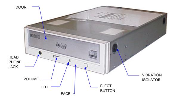
Fig. II - 1 Compact Disc Rewritable Auto Changer Drive configuration
