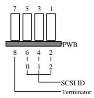
Fig. II - 6 Jumper Connector
