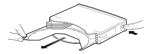
Fig. III - 6 How to eject/insert CDs from/in the magazine
