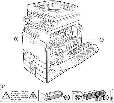
Do not touch the parts a label indicates. The inside of the machine could be very hot. Caution should be taken when removing misfed paper.
