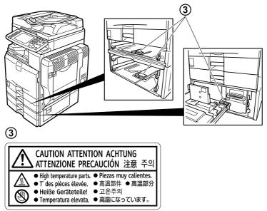
The inside of the machine could be very hot. Do not touch the parts which a label is put on. Otherwise, an injury might occur.
