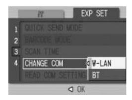
To send files by wireless LAN, you must use the computer to create a communication list registering the advanced settings for sending files, and then transfer the communication list to the camera. Use the provided Caplio Setting software to make the settings.
