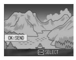
Once the transfer is completed, the camera returns to shooting mode and remains connected to the destination device. You can change to playback mode or voice memo mode or remain connected to the destination device until the camera is turned off. The Bluetooth<sup>®</sup> antenna icon appears on the LCD monitor while the camera is connected.
