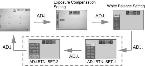
The screenshots above are examples of the screen display when functions are assigned to [ADJ BTN. SET.1] and [ADJ BTN. SET.2]. Press the ADJ. button until the screen with the desired function appears. Adjust the settings with the  $\blacktriangle \blacktriangledown$  buttons and press the MENU/OK button to set.
