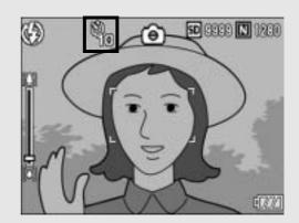
• Each press of the 🕲 (Self-timer) button changes the self-timer setting in the following order: 10 sec, 2 sec, and Self-timer Off.
