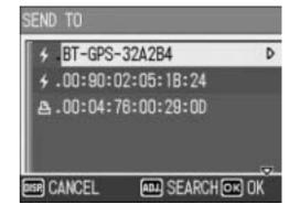
• To delete a destination device from the list, select the device and press the Ⅲ (Delete) button.
