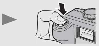
• The still image you have taken appears momentarily on the LCD monitor and is recorded to the internal memory or SD memory card.
