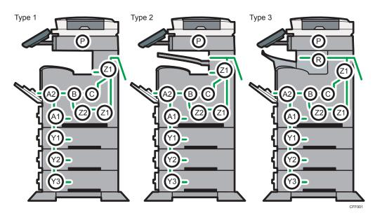
1. Press the key of the section from where you want to remove the jammed paper.
