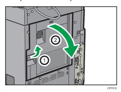
2. Release the lock of the fusing unit.
