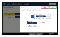
You can specify the printing position between -5.0 mm to 5.0 mm in increments of 0.1 mm.
