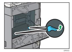
3. Pull out the fusing unit.
