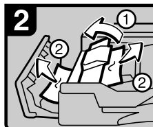
2. Remove misfed originals. 3. Close the cover P1 of the ADF. 4. Lift and lower the ADF.
