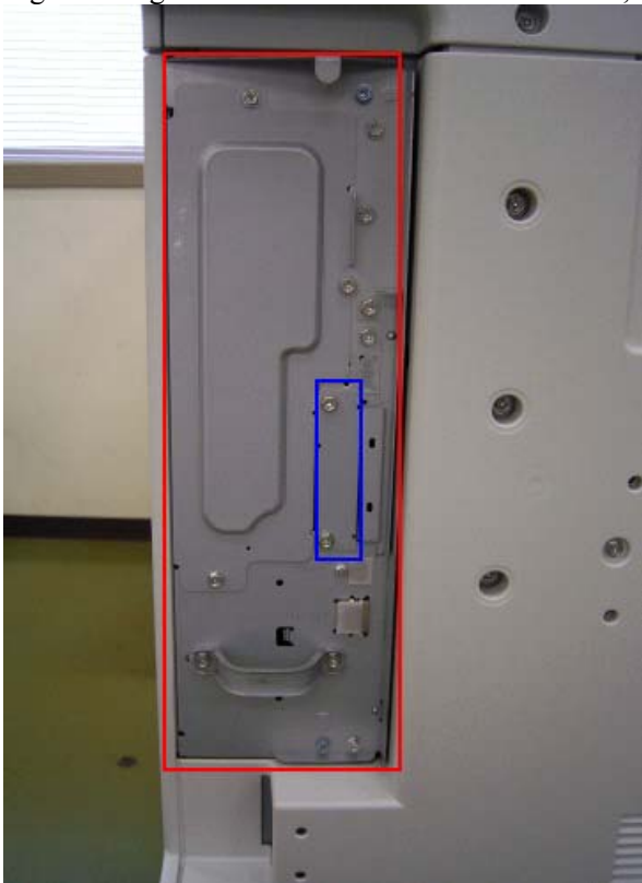
Fig 2. Enlarged view of Location of “R-WL54MG, R-WL54CG” to be equipped for a printer (example)
