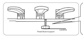
Before moving the piano to a new location, always remember to raise the level of the Pedal Board support so that it is not touching the floor. Once the piano is in place, you can adjust it so it is in firm contact with the floor again.
