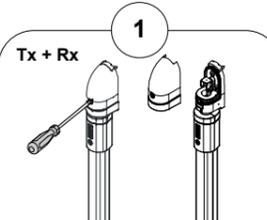
**EN** Open and pull out the tamper covers on the top and bottom of both the Tx and Rx rails.
